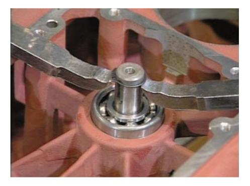
To remove the output shaft remove the circlip on gear side V using cranked circlip pliers. Support the worm wheel against the gear housing with matched support stops and then press the output shaft out in the direction of gear side H.
